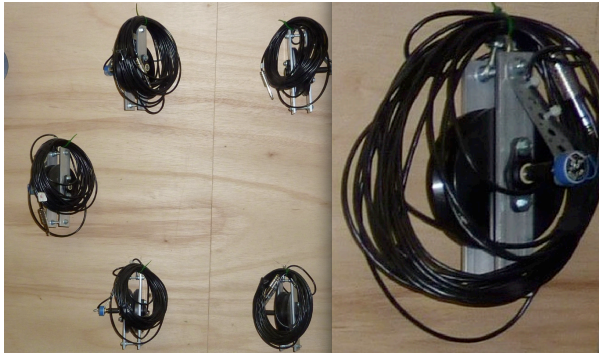
Figure 2. Sensors consisting of wheels, housing, cabling and potentiometers (in blue in the upper right corner detail)
