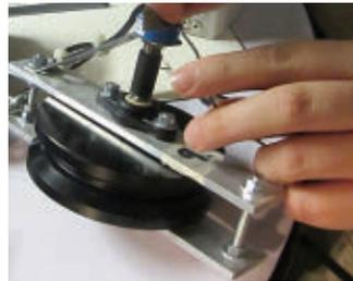
→ One of eight sensors, consisting of wheel, housing, cabling, and potentiometer.
